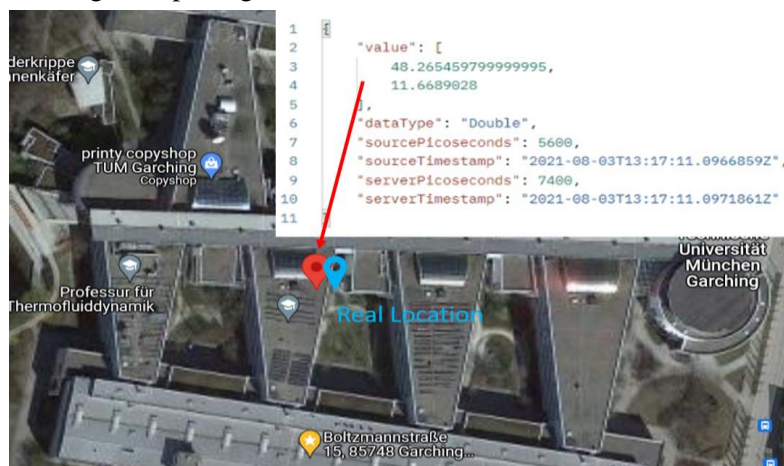
Fig. 7: GPS data requested through OPC-UA API Gateway
