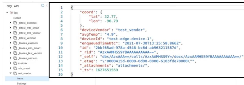
Fig. 4: Data collection in the centralized CosmosDB.
